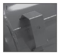
bottom of the rubber foot (Fig.2), then through the foot mounting hole on the compressor, and fasten using the corresponding nut.
